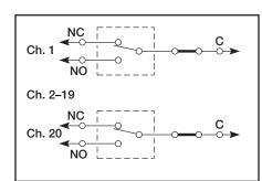
CHANNELS PER CARD: 20 independent Form C. All poles available at connectors. Replacement of factory installed jumper allows current limit resistor in series with common of each channel. On-card bus allows for addition of jumper to change configuration from switch to multiplex. Bus also allows channel interconnection.
